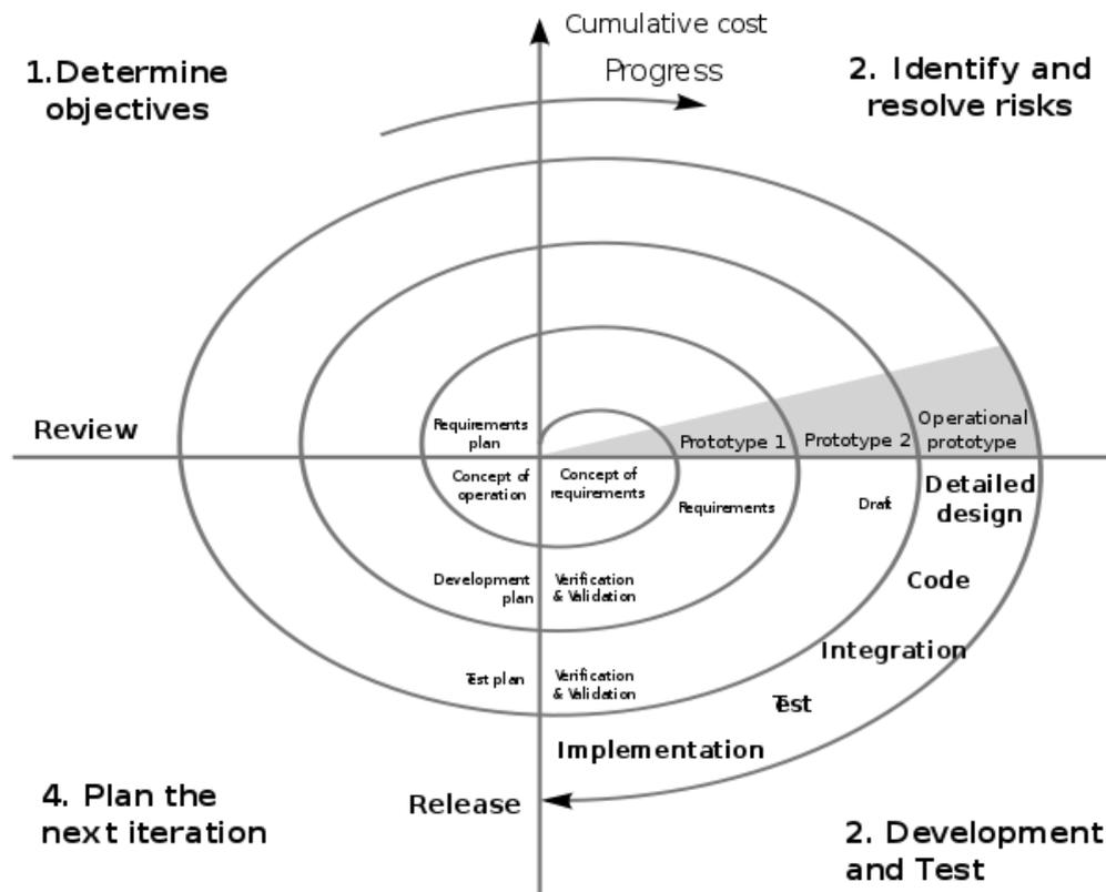
Figure 3. The steps of software development based on Spiral model. Source: (Boehm, 1986).
