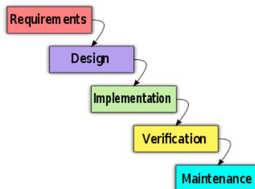
*Figure 1. The steps of software development process based on waterfall model. Source: (Wikipedia, 2010a).*
