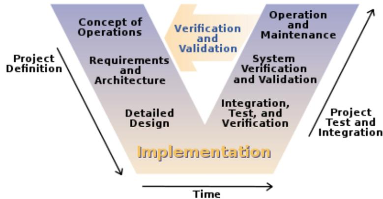
Figure 2. The steps of software development based on V-shaped model. Source: (FHWA, 2005).
